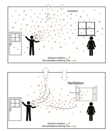
Distribution of respiratory microdroplets in an indoor environment with (A) inadequate ventilation and (B) adequate ventilation.
